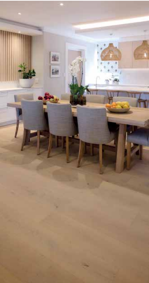
COVER IMAGE: FINOAK 15/4 190MM CLEAR GRADE WITH A GHOST WHITE CUSTOM OLEUM STAIN AND 2K SEALER TO CLIENTS SPECIFICATIONS
